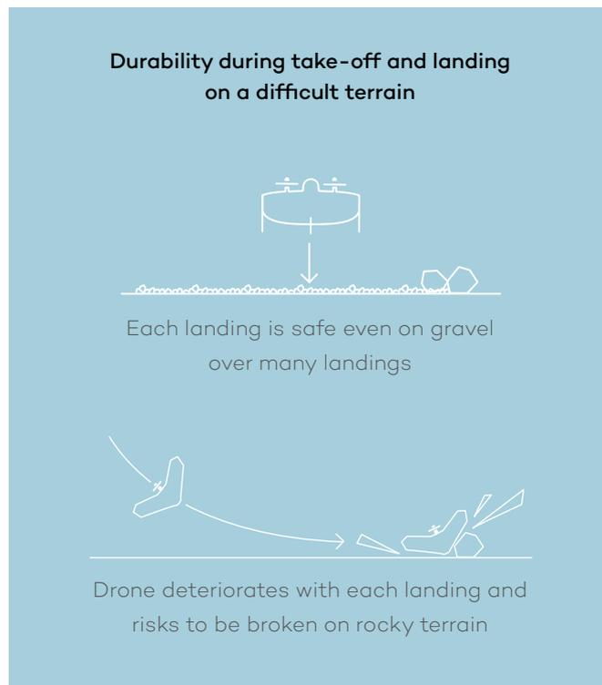
Smooth vertical landing guarantees not only the safety of the drone but also of its onboard high-end sensor. Belly landing drones are unable to carry sensors of similar quality due to the increase in weight and harder skid landings.
